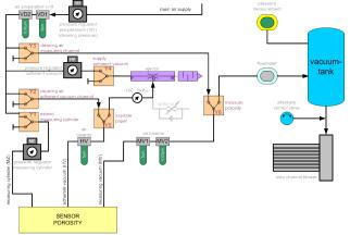
Both quantities calculated result in a value for the air permeability of the measured material.
