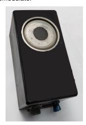
The sensor only requires a 24V supply voltage from the outside. The sensor output signal is available as Profibus DP signal.
