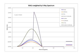
If several combinations of fillers are operated in one system, the X-ray voltage must be adjusted according to the recipe. In addition, the corresponding filters are placed in the X-ray channel to create the condition of the same MAC's.
